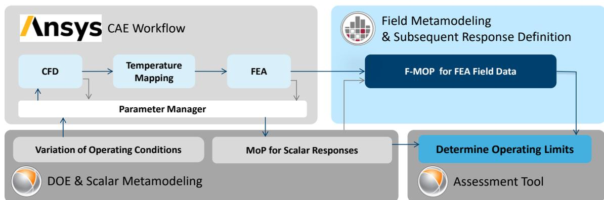
Figure 5: Example of Rheinmetall Automotive Workflow for subsequent Response Definition
